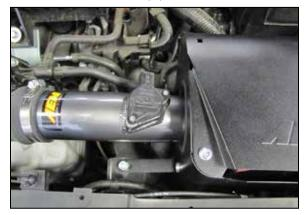
11. Remove the mass air sensor from the factory air filter housing and install the mass air sensor into the AEM<sup>®</sup> intake using the provided hardware.
