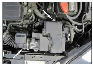
4. Remove the two bolts that secure the factory air filter housing. Pull up the filter housing and remove it from the vehicle.
