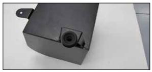
6. Remove the mounting grommet from the factory air filter housing and install it into the AEM<sup>®</sup> heat shield as shown.
