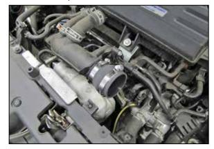
9. Install the provided coupler (084018) onto the turbo inlet tube and secure with the provided hose clamp.
